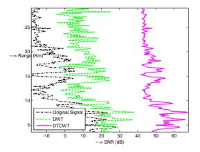
Fig.2 SNR Comparison in Zenith-x direction
